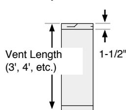
Vent Height is calculated to the top of the vent on horizontal terminations and to the top of the termination on vertical terminations.
