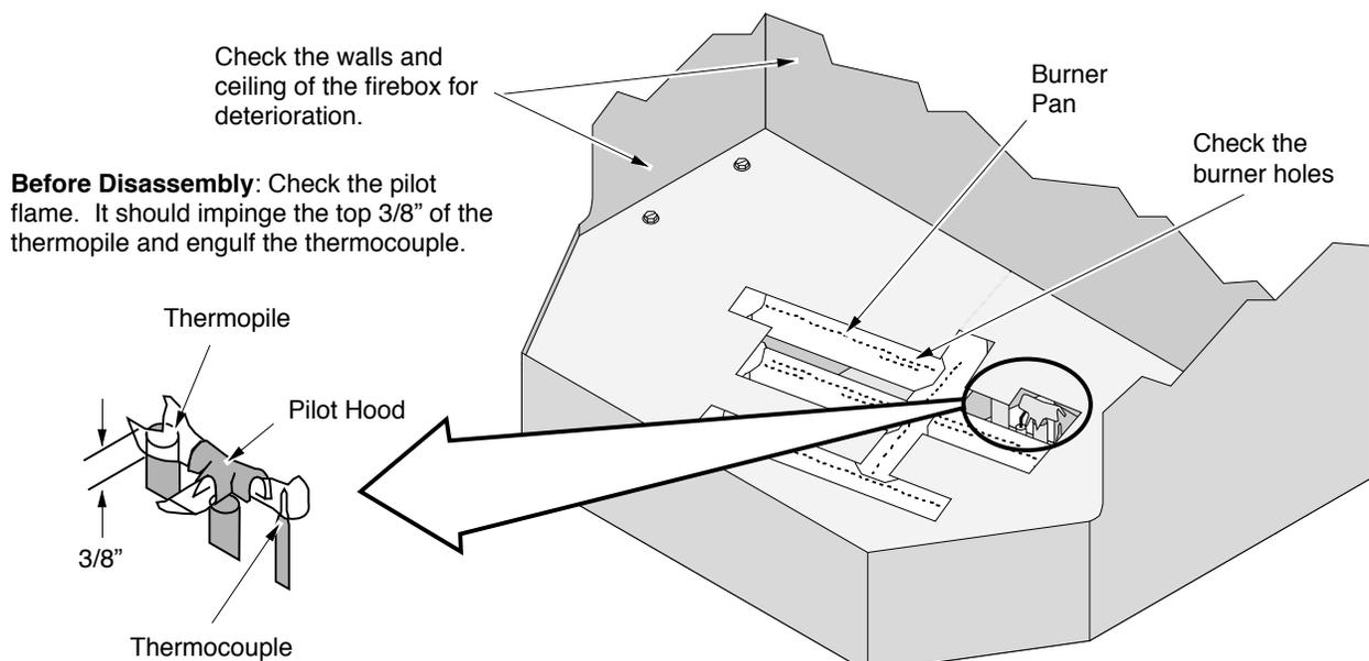
**Before Disassembly:** Check the pilot flame. It should impinge the top 3/8" of the thermopile and engulf the thermocouple.
