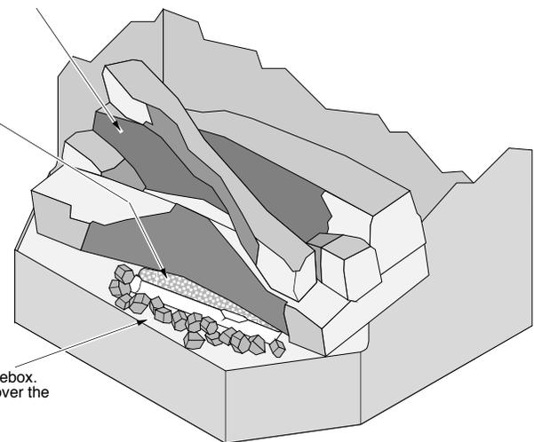
Place the kibbles in front of the firebox. Do not place the kibbles directly over the burner holes.
