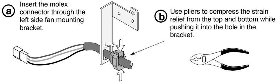
6 Install the blower assembly following the directions below.
