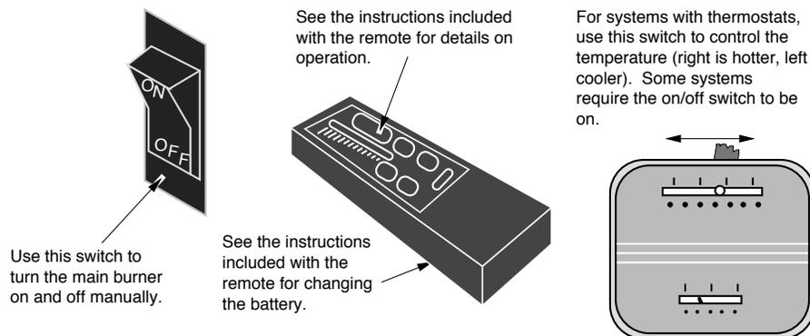
**Warning:** Do not place combustible items on top or directly in front of the heater, even temporarily. The optional thermostat may start the heater causing a combustible item to ignite.
